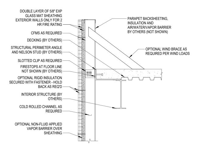
REFERENCE DETAIL ONLY - CONSULT WITH CFMS STRUCTURAL ENGINEER FOR SIZING, BRACING AND ATTACHMENT REQUIREMENTS
