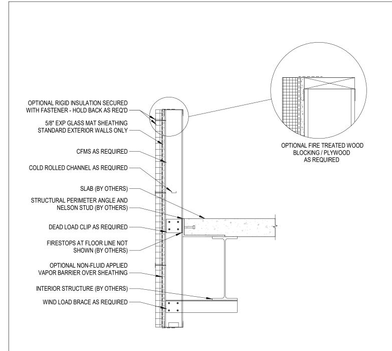
REFERENCE DETAIL ONLY - CONSULT WITH CFMS STRUCTURAL ENGINEER FOR SIZING, BRACING AND ATTACHMENT REQUIREMENTS
