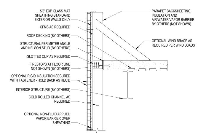
REFERENCE DETAIL ONLY - CONSULT WITH CFMS STRUCTURAL ENGINEER FOR SIZING, BRACING AND ATTACHMENT REQUIREMENTS
