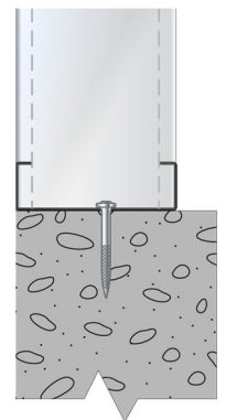
Powder Actuated Fasteners to Foundation
